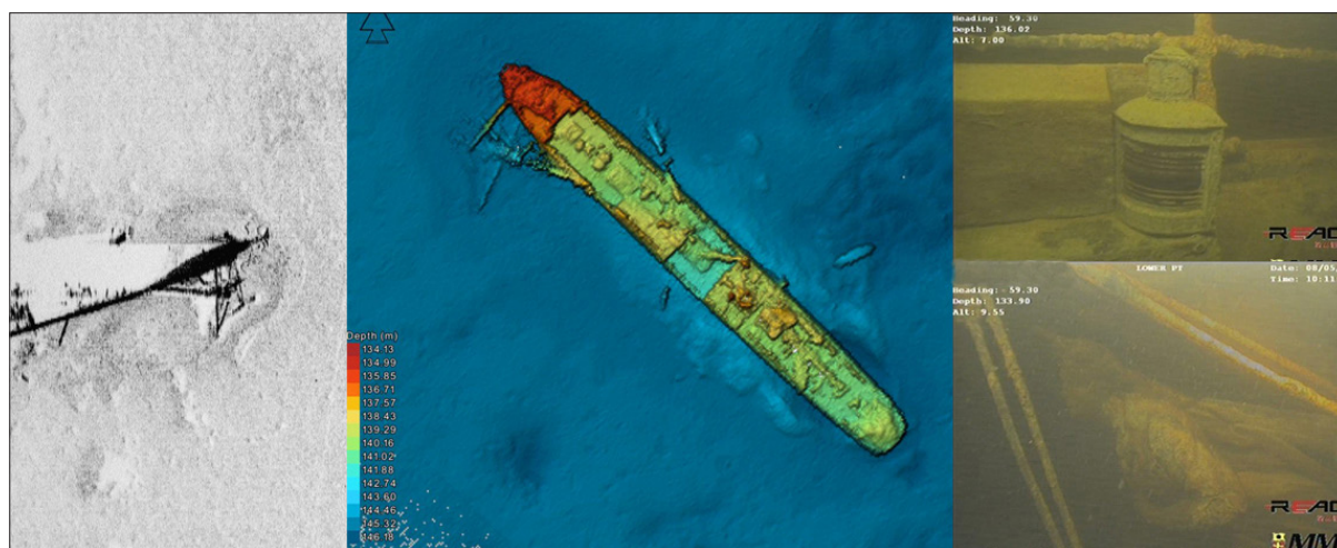
Fig. 11. Sonar image, multibeam image and photos of port navigation light and bow figure head at S-R24-5317 © Fugro and MMT.
