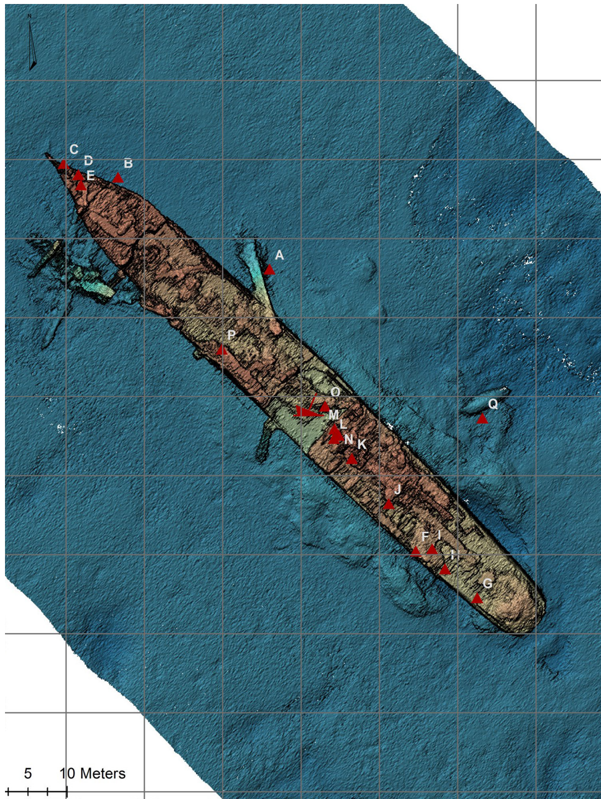
FIG. 20. Multi-beam image of wreck S-R24-5317. MMT "Events A-Q. A: Collapsed mast of the wreck, B: Figurehead, C: Anchor on the main deck, D: Bow of the wreck, E: Main deck of the shipwreck, F: Debris item, a cup, G: Port hole, H: Wooden ladder, I:Upside down life boat on the main deck of the wreck, J: Part of a chimney, K: Steel frame windows, L: Ship's bell, M: Compass, N: Davit (Machine telegraph) , O: Wooden steering wheel, P: Port navigation light, Q: Upside down life boat to the starboard side of the wreck. MMT/Nord Stream 2.
